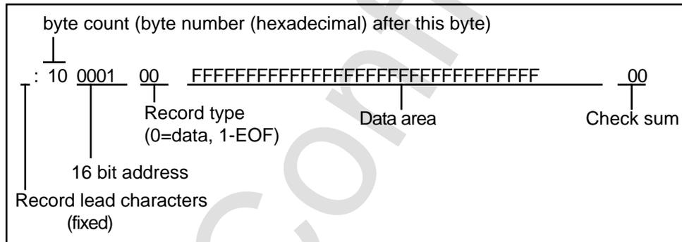
The check sum is a complement of double binary addition as far as the byte immediately before check sum within the code that contains the byte count, address, record type, and data.
