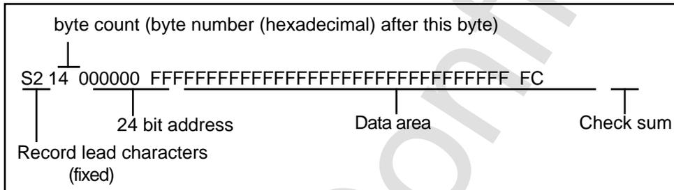
The check sum is a complement of single binary addition as far as the byte immediately before check sum within the code that contains the byte count, address, and data.
