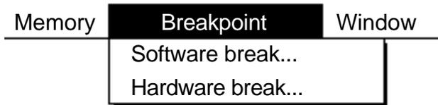
When selecting **Software Break**, the following movable modal dialog box will be displayed: The same operations as can be performed by the console commands **B**, **BE**, **BC** and **BR** can be performed.
