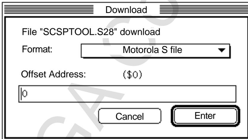
3. The format is set in a menu, and the offset address is set by inputting a formula.
