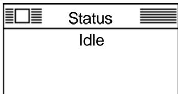
However, when a break is not applied without reaching the pass count with software breaks, an idle display or debugger program PC display may temporarily appear even when the user program is normally being executed.
