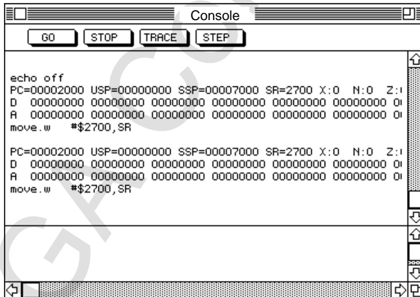
The four buttons at the top of the window have a one-to-one correspondence with the console commands as shown below, and when a button is clicked, the respective console command is entered.
