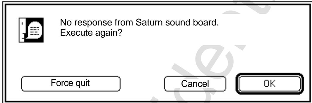
If the sound board should hang up at this time, the SCSI bus is taken over and stopped, thus hanging up the Macintosh as well. This happens when display of the message (in the dialog box) "No response" is attempted, the resource cannot be read in because the SCSI bus has been taken over, thus resulting in a window being displayed with nothing in it and hanging up the system.
