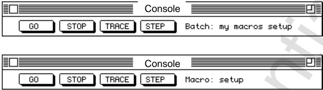
The bottom part of the window is the input area. This is normal edited text, so cut and paste can be used freely. The result of execution of console commands is displayed in the area between the input area and the buttons at the top. A backlog of results can be viewed by using the scroll bar.
