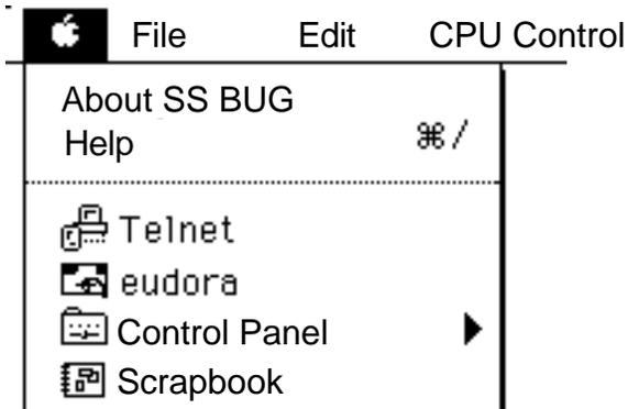
“**About SSBug...**” displays the version and other information about SSBug. The window is closed by clicking in the window.
