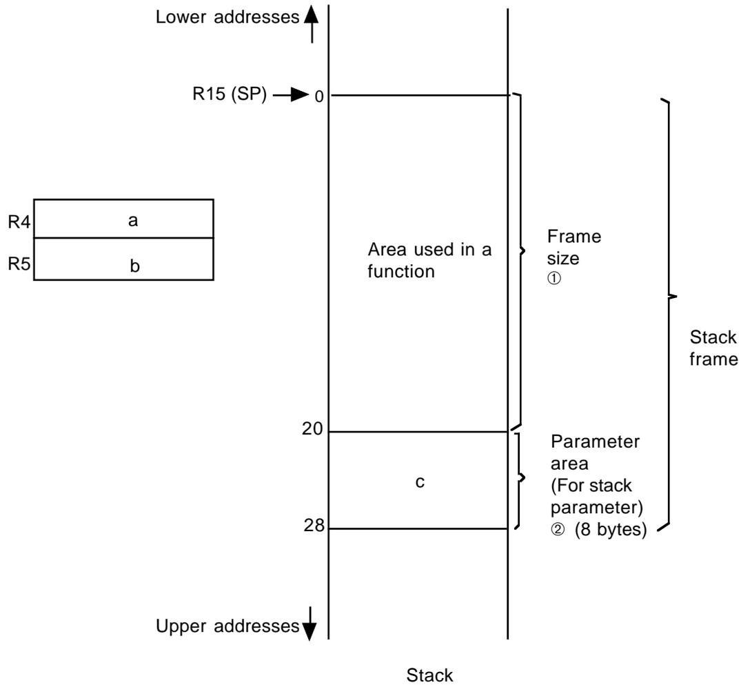
The size of stack used by a function is determined by adding frame size and parameter area size (for stack parameter). Accordingly, in the above example, the stack size used by the function is calculated as follows: 20 (①) + 8 (②) = 28 bytes
