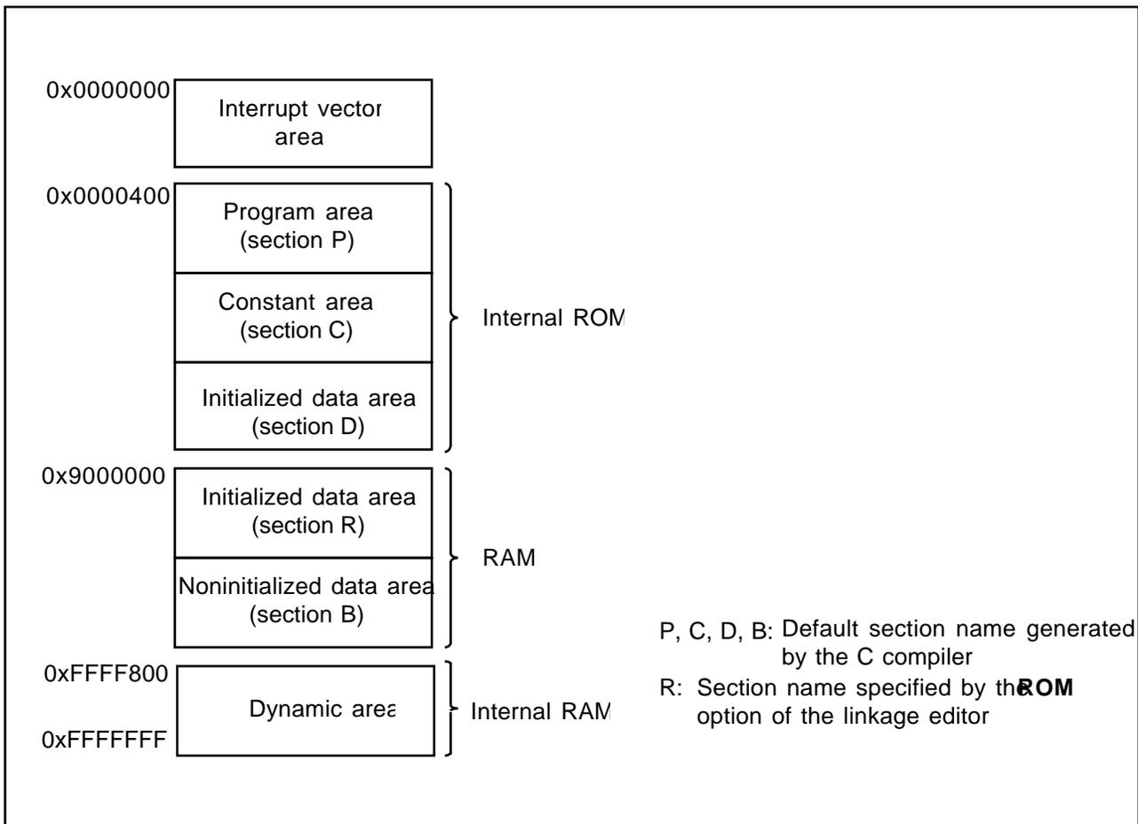
**Figure 2-2 Static Area Allocation**
