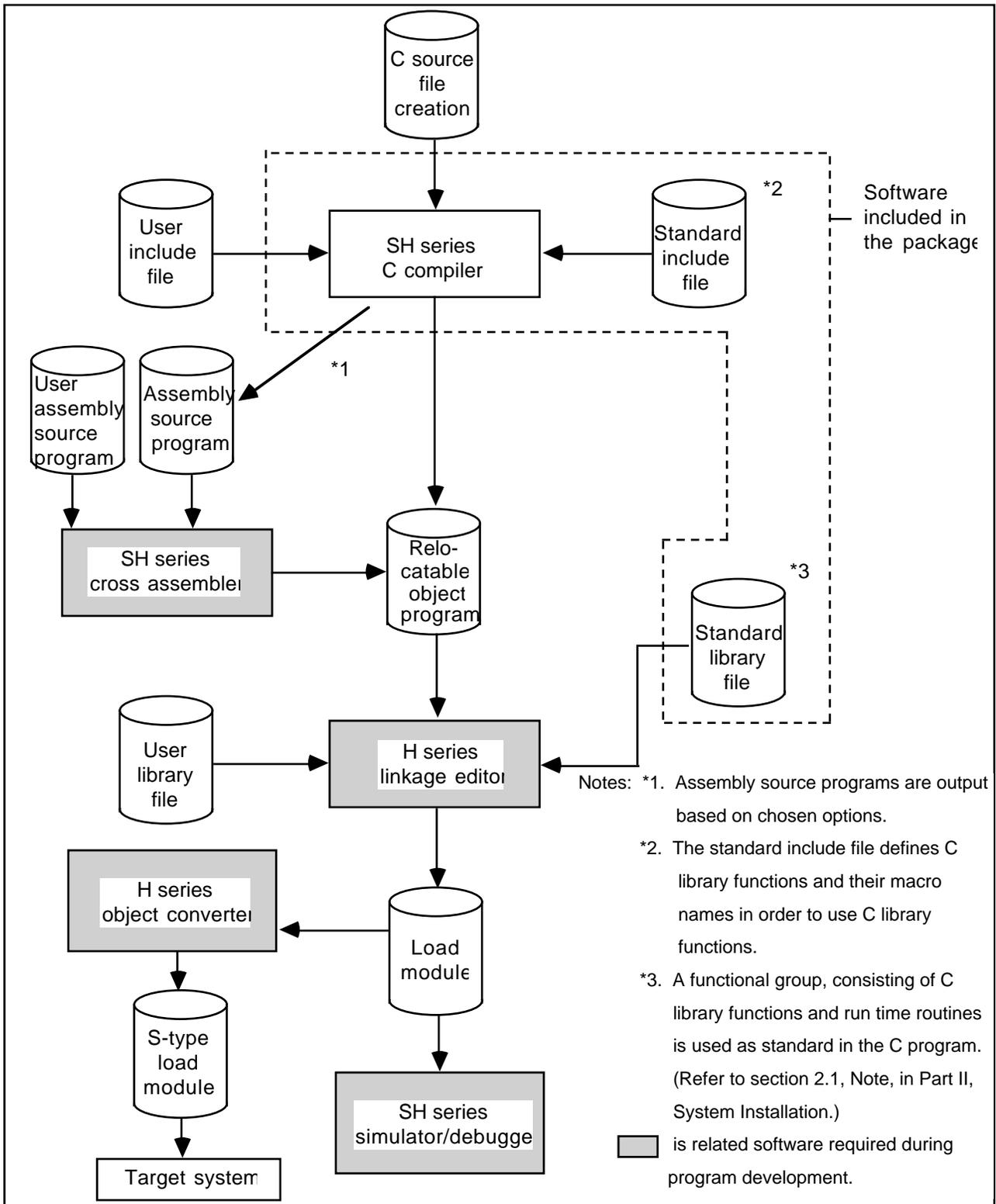
**Figure 2-1 Relationship between the C Compiler and Other Software**
