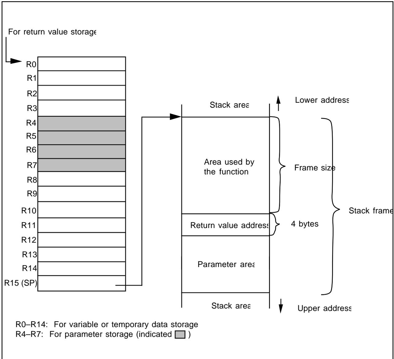
Figure C-1 Usage of Registers and Stack Area
