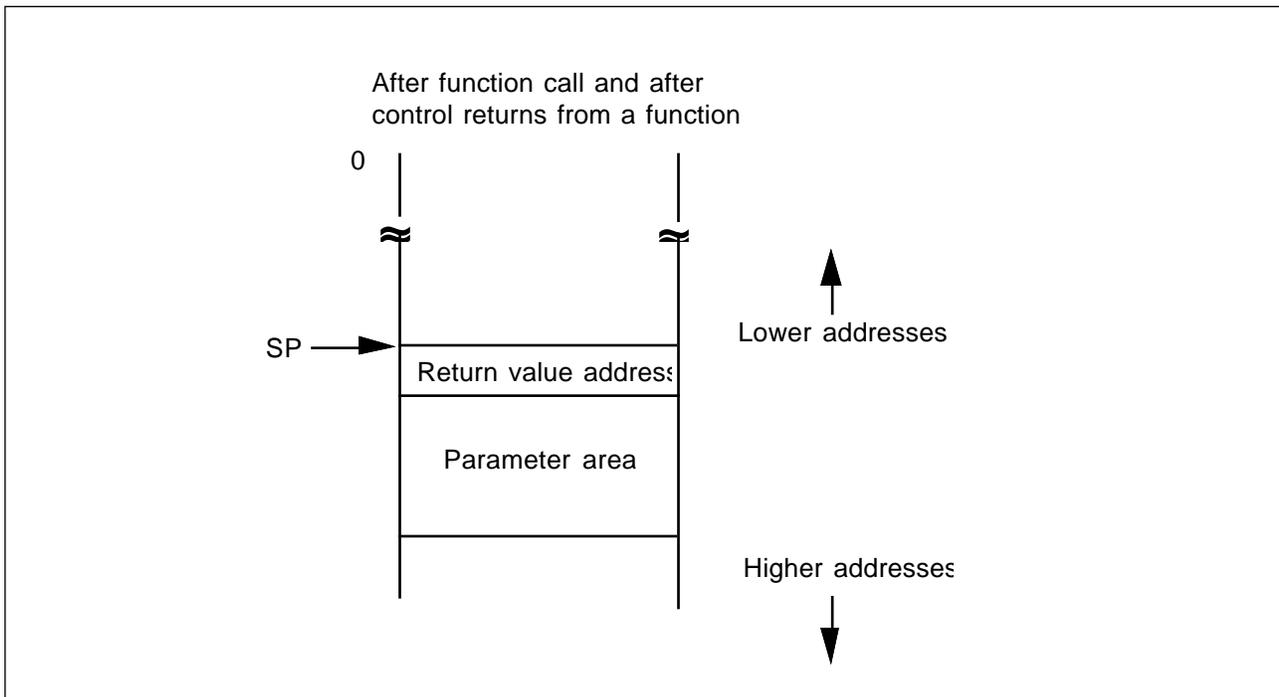
**Figure 2-1 Allocation and Deallocation of a Stack Frame**
