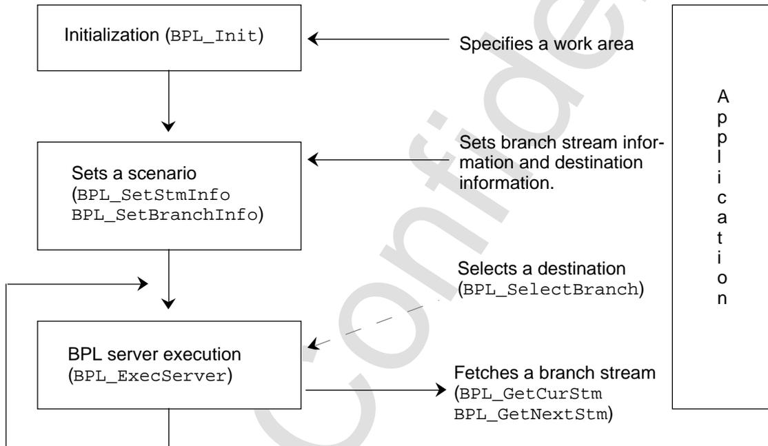
Figure 3.1 Flow of processing
