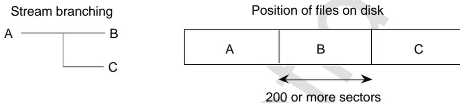
**Figure 4.1 Non-interleaved candidate branches (C cannot be pre-read)**
